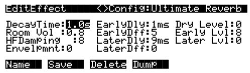
The top line tells you that you're in the Effects Editor, and identifies the configuration (explained below) of the currently selected preset effect. The bottom line labels the active soft buttons. The parameters you see depend on the currently selected configuration.
